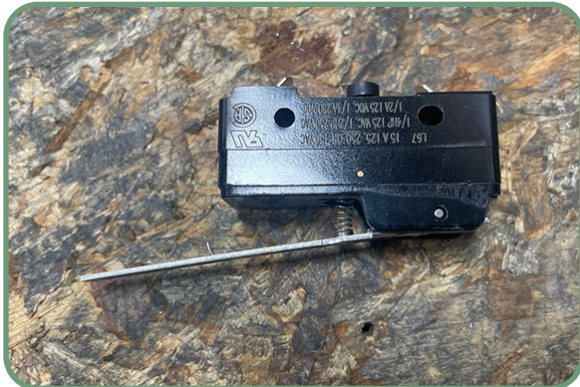
94033 - Switch, Man. Reset (slack cable)
